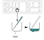
Pipette slowly into the bottom of the reservoir where the inlet is located. Raise the pipette tip as the liquid level in the reservoir is rising, keeping the tip slightly submerged.
