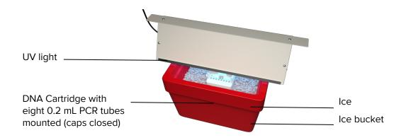
5.2 Place a UV light on top of the ice bucket and **expose the samples to UV light for 8 minutes.** The distance between sample and UV light must not exceed 5 inches.
